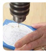
have the space, use a larger bit—it will make it easier to thread the blades through. For thin veining cuts, use the smallest bit the blade will fit through.
