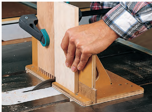
After the last cut , clamp this piece to the jig fence and use it to index the first cut on the mating part, as shown in the right photo, above.
