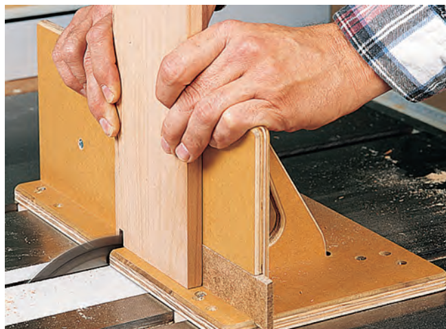
Once the pin is adjusted properly , the first series of pins and slots can be cut across the first workpiece (left photo, above).
