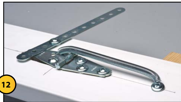
12 Stretch the spring and attach it to the bottom of the track.
