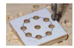
Drill the center hole and tooth valleys with brad-point bits as marked on the patterns.
