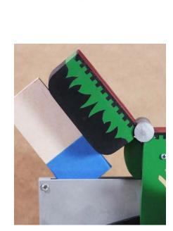
▲ Step 16: Attach the top of the head. While the cantilevered head top might look precarious, a little preparation and the right glue will ensure a rock-solid connection. Wrap a scrap of plywood with a single layer of painter's tape, and then wedge it into the screen opening with the head resting on the top of the ears. Apply two-part epoxy to the "hinge" socket to seal the deal.
