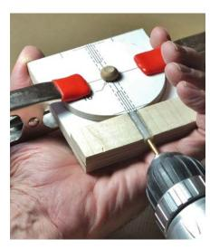
▲ Step 6: Drill the holes in the rotor disc. Use the same jig and drilling
