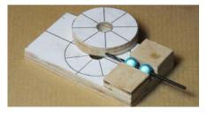
▲ Step 9: Make the bead gear jig. The plastic beads that will eventually
