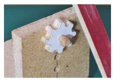
File and/or sand any irregularities on a holding fixture with a 5/16" (8mm)-diameter axle inserted through the axle hole. Do not remove the sacrificial backer until you've completed this refinement process. Note: The "files" that I find most useful for this step are large, homemade emery boards. They're strips of 1/4" (6mm) Baltic birch plywood faced on alternate sides with 80- and 180-grit sandpaper.
