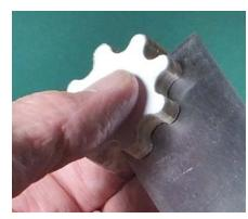
When you're satisfied with quality of your work, separate the finished gear from the sacrificial backer with a sharpened metal putty knife. Don't try to pop them apart. A gentle sliding motion is all that's required.
