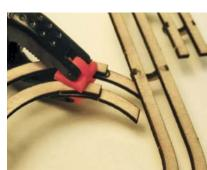
the under side of the outside track, clamp or weight, and let dry. Repeat for the inside joiner (marked I). Sand the transition smooth. Then, glue and clamp the track to the lower and side track supports. Let
