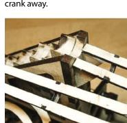
The cam-driven steps elevate the marbles to the top of the track, and gravity returns them to the base of the steps.
