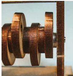
Place three or four washers on each end of the camshaft to achieve a proper fit between the frame uprights (Step 3).
