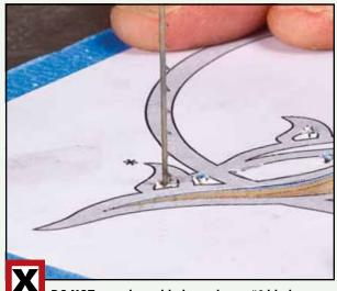
**DO NOT** use a large blade, such as a #9 blade, to cut intricate designs in thin wood. The large blade cuts thin wood too quickly, does not fit into tight areas, and can be difficult to control.
