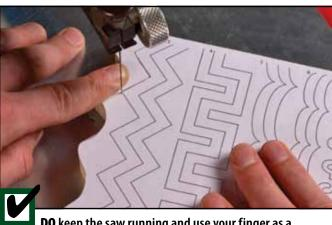
**DO** keep the saw running and use your finger as a pivot point. Position your finger behind the blade, apply pressure, and use the finger as a pivot point. Use the opposite hand to rotate the blank. With practice, you can turn the blank without hearing the blade cut any wood.
