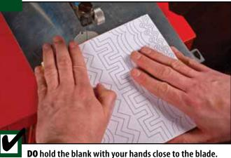
DO hold the blank with your hands close to the blade I position my pinky and thumb on the edge of the blank if possible. This grip provides the most control and prevents the blank from chattering as the action of the saw bounces it off the saw table.
