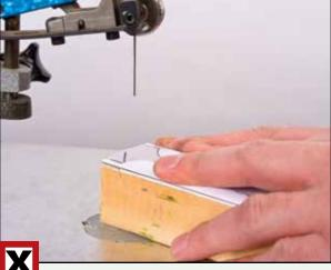
DO NOT use a small blade, such as a #3 blade, to cut wood more than 3/4" (19mm) thick. The small blade will dull quickly, burn the wood, and break prematurely.
