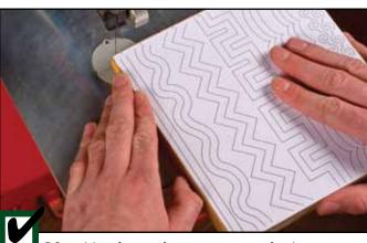
**DO** position the wood so your stronger, dominant hand controls the largest part of the blank. If you are right-handed, the majority of the wood should be positioned on the right side of the blade.
