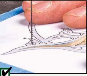
DO use a small blade, such as a #3 blade, to cut **intricate designs in thin wood.** The small blade cuts slower than a large blade, fits into tight corners, and is easier to control.
