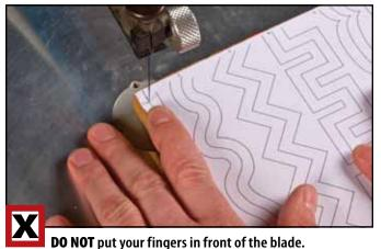
Demonstrators often place their finger on a moving scroll saw blade to show how safe the saws are, but if your finger is held against the wood when you touch the blade, you can get a small slice.
