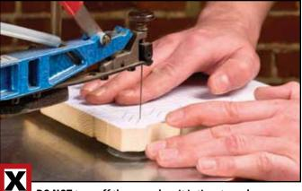
DO NOT turn off the saw when it is time to make a sharp turn. When you turn the saw back on, it will catch the blank and slam it back down onto the table, possibly breaking your work or pinching your finger.
