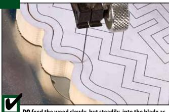
**DO** feed the wood slowly, but steadily, into the blade as you cut the curve. The more you can keep the feed rate constant, the smoother the overall cut and shape of the curve will be.
