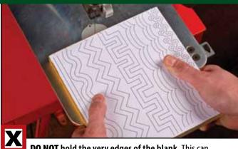
**DO NOT hold the very edges of the blank.** This can cause you to lose control of the cut as your turn a corner.
