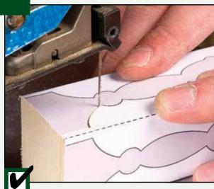
DO use a large blade, such as a #9 blade, to cut thick wood. The large blade clears the sawdust better and cuts faster than a small blade without dulling, burning the wood, or breaking.
