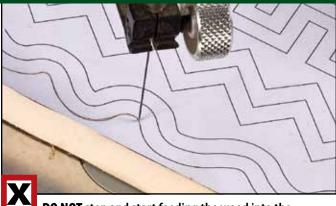
**DO NOT** stop and start feeding the wood into the blade as you attempt to cut a circle or sweeping curve. This will produce a rough and choppy edge.
