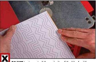
**DO NOT** try to control the majority of the blank with your non-dominant hand. It will be difficult to control the blank if your weaker, less-coordinated hand is doing most of the work.
