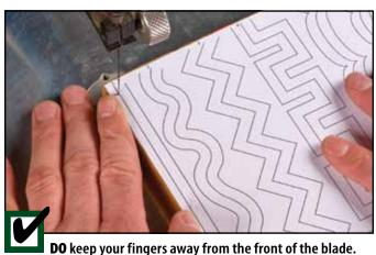
You can have your finger in front of the blade as long as it's a good distance from the blade, but a better position is to have your fingers about an inch away from the side of the blade when possible.
