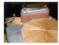
▲ **Step 6**: **Sand the tabletop.** Using a belt sander, sand the outside edges of the top. Then, sand the top and bottom portions to achieve a flat surface.
