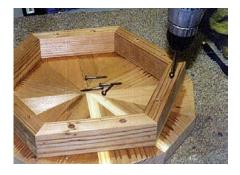
▲ Step 10: Prepare the screw holes. Set the assembled and sanded apron on the underside of the tabletop. Referring to the assembly drawing, mark the screw hole mounting locations. Countersink a ¾" (10mm)-diameter by 1" (25mm)-deep hole for each screw in the bottom edge of the apron.
