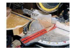
▲ Step 4: Cut the second angle. Set the miter saw to a 15° angle. Make a mark 1" (25mm) from the corner, place the square edge of the piece against the saw fence, and cut along the line to remove the sharp edge.
