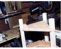
▲ **Step 19**: **Fill the holes.** Use pieces of ¾" (10mm)-diameter cherry dowel rod to fill the countersunk holes on the outside legs. Glue, cut them off flush with the edges of the legs with a hand saw, and sand.
