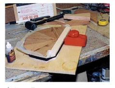
▲ Step 5: Glue and clamp the sections. Using waterproof glue, assemble and clamp six pieces together to create half of the tabletop. Use a web clamp against a sturdy piece of wood scrap to apply pressure, and use waxed paper to make sure the glue stays on the pieces. When the glue has cured, assemble the other half. Connect the two halves using glue, the web clamp, and other clamps as needed.
