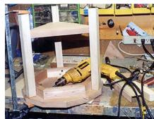
A Step 16: Drill leg holes. Drill a ¾" (10mm)-diameter by ¾" (10mm)-deep countersink hole on the outside of each leg, across from where it mates with the shelf. Then, drill two ¾" (10mm)-diameter by ¾" (10mm)-deep countersink holes on the inside of the apron across from each leg location.
