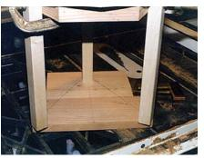
▲ Step 14: Check the leg placement. Temporarily clamp the legs to the apron. Set the assembly on top of the shelf to ensure the proper placement of the legs on the shelf.
