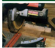
▲ Step 1: Cut the pieces to size. To cut the tabletop pieces, plane both sides of three 16" (406mm)-long pieces of redwood to 1" (25mm) thick. Joint one edge and rip the wood to 4½" (114mm) wide. Crosscut the pieces into six 8" (203mm)-long pieces.
