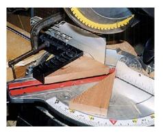
▲ Step 2: Cut the pieces on an angle. Set a miter saw to a 30° angle. Make a diagonal cut from corner to corner on an 8" (203mm) side of the tabletop pieces. Clamp a corner brace or square blank to the fence to secure the stock and keep your fingers out of the way.
