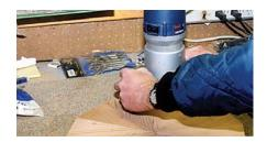
▲ **Step 7**: **Round over the edges.** Install a ¼" (3mm)-radius round-over bearing bit in a router. Round the top and bottom edges of the tabletop.
