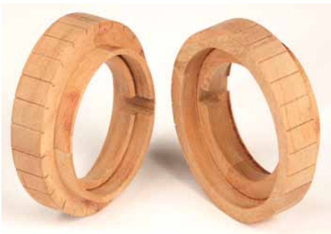
A view of the male and female ends of the rotating rings. The notches cut into the inside of the rings make a keyway for the pins to follow.
