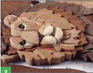
2 Sand the edges of the pieces on risers. This starts the process of blending them with the lower pieces beside them. Use a 100-grit drum sander to remove material quickly. Once you rough in all of the levels, use the 220-grit drum to soften the edges and remove any scratches. Use pliers to hold the smaller pieces and wear finger protection when holding them. Mark the level on a piece and sand down to the line. Always keep the line side up and in sight. Replace the pieces onto the work board to see how each piece looks next to the surrounding pieces. Continue sanding until the entire lion is done.
