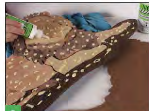
9 Trace the assembled project onto the backing board and cut it out. Apply dots of CA glue and wood glue to the back of the intarsia and apply accelerator to the backing board. Press the two together and trim off any overhanging backing board.
